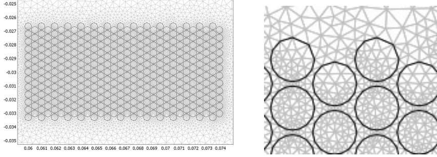
FIG. 2.2. Windings of the coil and FE mesh
