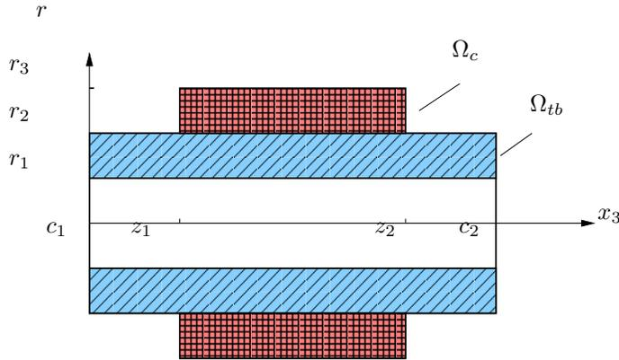
FIG. 2.1. Scheme of the tube with coil – cut through the origin along the  $x_3$ -axis
