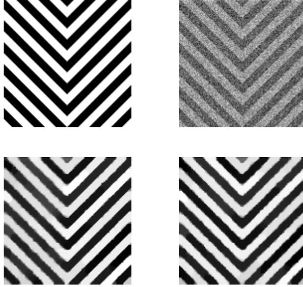
**Fig. 4.** Top left: Original image with values in  $[0,1]$ . Top right: Noisy image with white Gaussian noise of standard deviation 0.4. Bottom left: Denoised image by the ROF-model and forward difference discretization. Bottom right: Denoised image by the ROF-model and Haar filter discretization.
