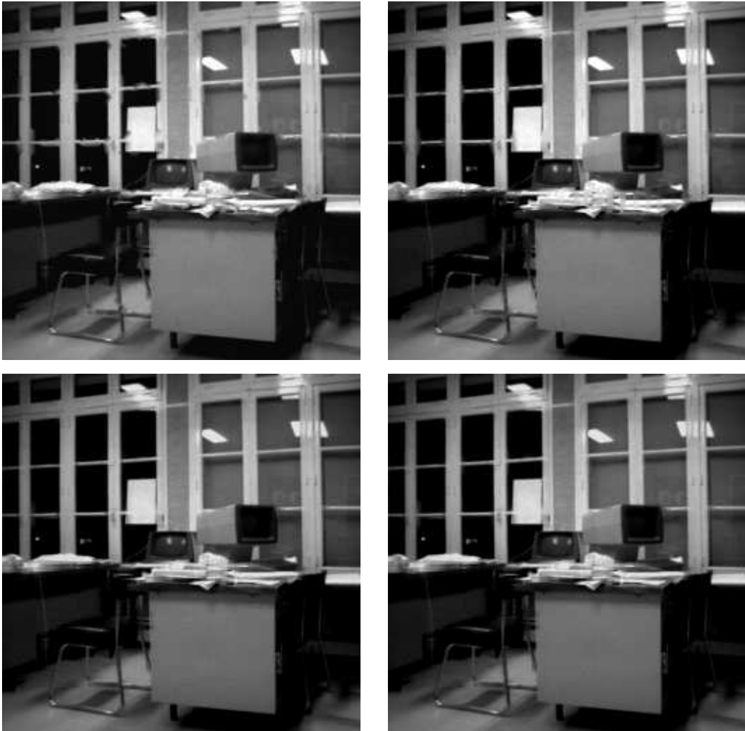
Figure 4: Interpolation of the image in Fig. 3. Top left: Cubic interpolation by the MATLAB procedure 'griddata' (PSNR=30.18, err_2 = 7.89 , err_1 = 1.51 ). Top right: algorithm A, (PSNR=31.61, err_2 = 6.69 , err_1 = 1.36 ). Bottom left: algorithm B, (PSNR=34.08, err_2 = 5.03 , err_1 = 0.93 ). Bottom right: algorithm C, (PSNR=33.98, err_2 = 5.09 , err_1 = 0.97 ). The images at the top contain artifacts, in particular at the left window side. The algorithms at the bottom show a better performance and do not introduce these artifacts.
