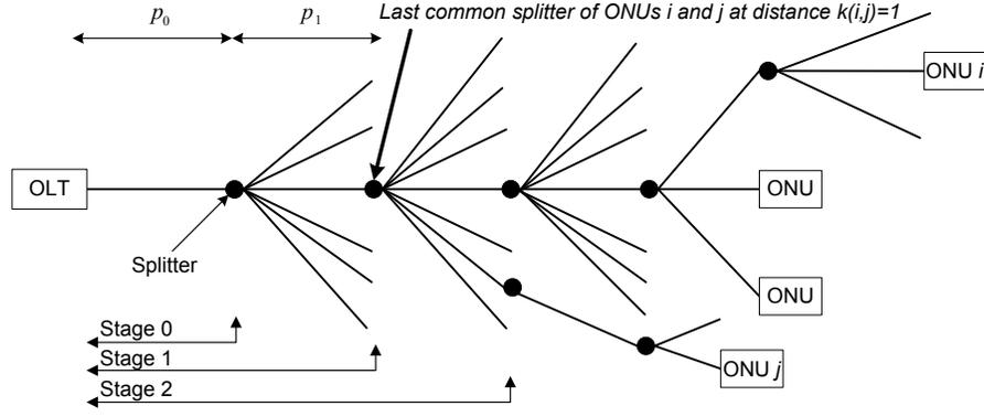
Fig. 4. LR-PON and last common splitter of ONU  $i$  and ONU  $j$  for  $d_i = 5$ ,  $d_j = 4$ , and  $k(i, j) = 1$ .
