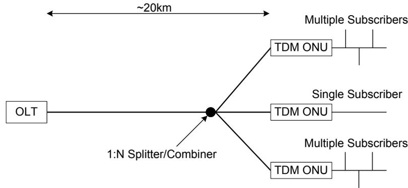
Fig. 1. Network architecture of a conventional TDM PON with one OLT and  $N = 3$  ONUs.
