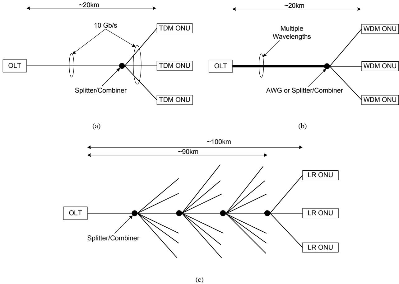
Fig. 2. Next-Generation Passive Optical Networks (NG-PONs): (a) high-speed TDM PON, (b) WDM PON, and (c) LR-PON.
