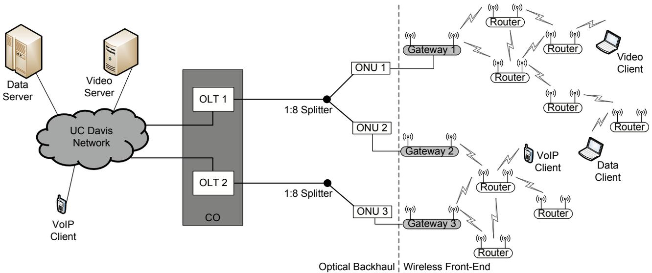
Fig. 3. R&F-based FiWi network: UC Davis R&F testbed integration of EPON and WMN [35].
