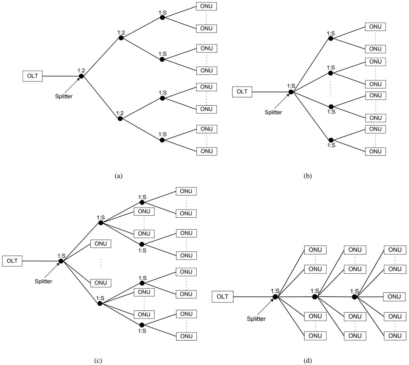
Fig. 7. NG-PON topologies: (a) binary tree, (b) full tree, (c) pyramid, and (d) cube.
