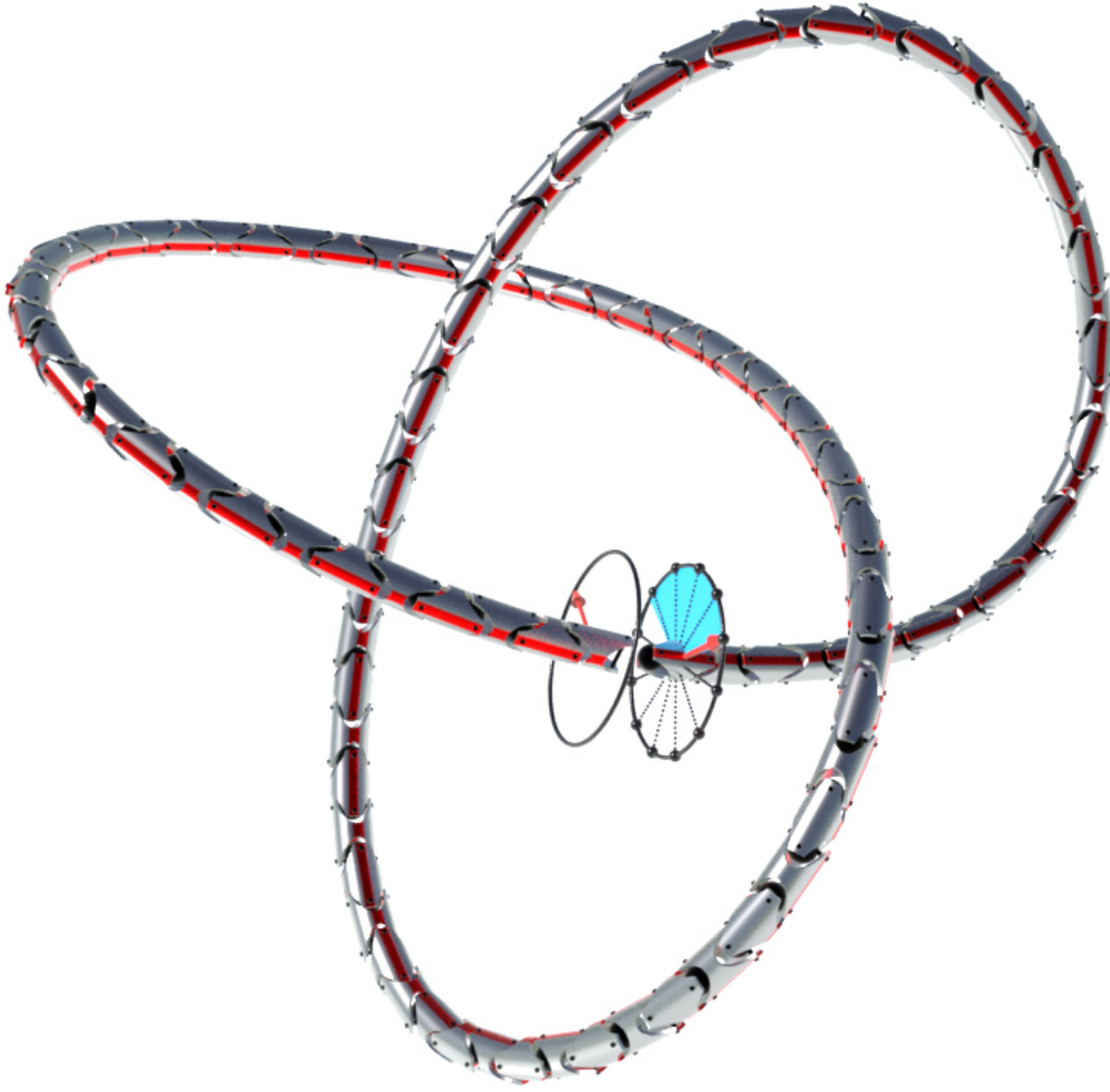
Figure 5.2. A trefoil knot cannot be built from constant-velocity joints. Because of the angle-defect due to the total torsion, the joints would not close up.
