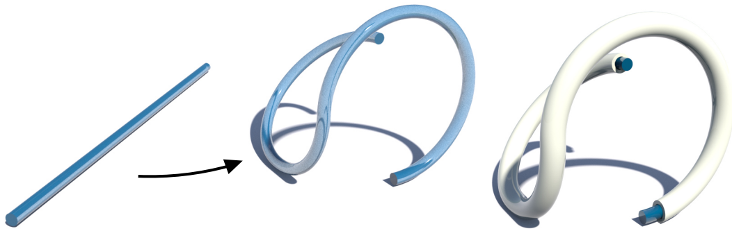
Figure 1.4. A rod is bent into the shape of a curve. Then it is fixed in its position by a porcelain case within which it can untwist while staying in shape.
