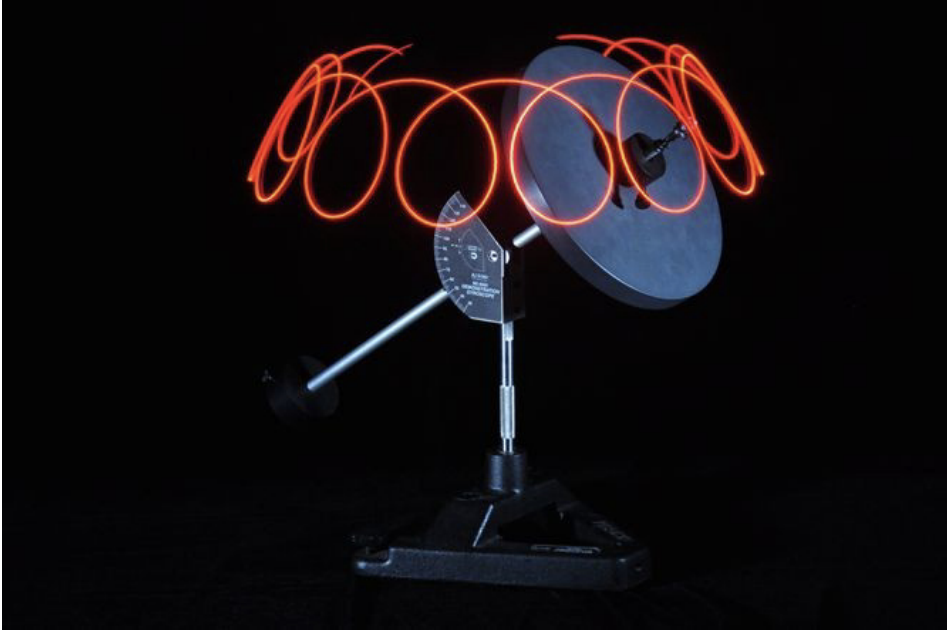
Figure 5.4. Kirchhoff showed that, as an elastic curve is traversed with unit speed, its tangent vector T follows the motion of the axis of a gyroscope. The photograph with long-time exposure: [41].
