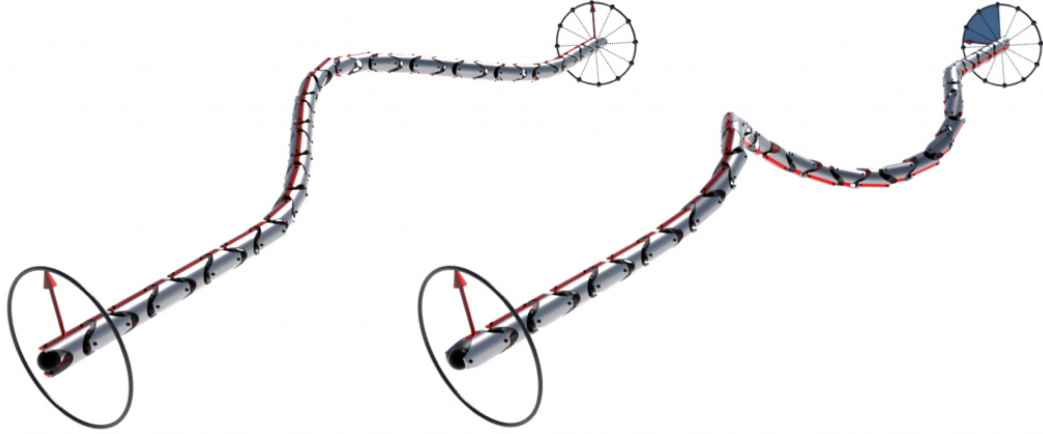
Figure 5.1. Two curves built from constant-velocity joints. The total torsion is zero for the curve on the left, but not for the one on the right. The red line indicates a parallel normal field.
