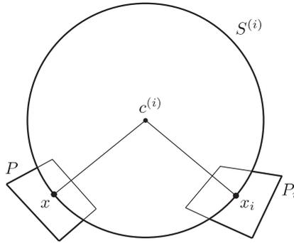
Figure 10. Principal-curvature sphere
