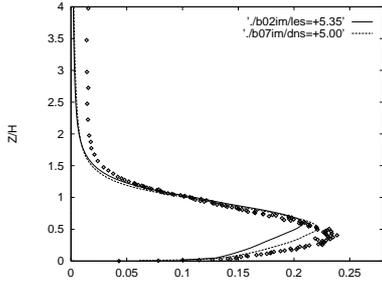
Figure 7:  $u_{rms}$  at  $x = 5H$
