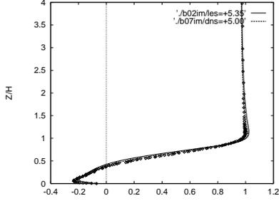
Figure 5:  $u_{mean}$  at  $x = 5H$
