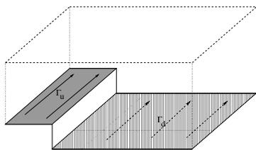
**Fig. 3.**  $\Gamma_u$  and  $\Gamma_d$  as a moving boundaries, with the lateral velocities  $v_u$  and  $v_d$
