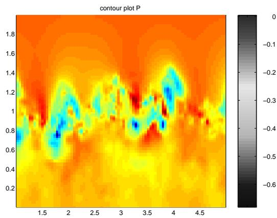
**Fig. 11.** pressure contours at  $x = 1 H$ , DNS
