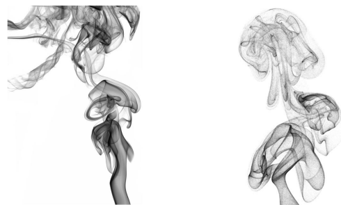
Figure 1: Comparison of a photograph (left, from [Jef]) with our simulation (right). The 396^2 particles are rendered as unshaded transparent GL points.
