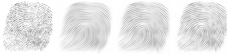
Figure 12: Left to right: (a) Fingerprint image, 100 \times 100 pixels. (b) Filtered with CED, \varepsilon = 0.001 , C = 1 , \sigma = 0.5 , \varrho = 4 , using the nonnegativity scheme [59] with \tau = 1/6 and N = 60 iterations. (c) Processed with our LSAS scheme ( \alpha = 0 ) for CED, same parameters. (d) LSAS scheme with \tau = 1 and N = 10 iterations.
