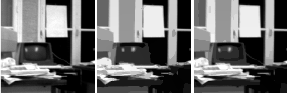
Figure 7: Left to right: (a) Original image from Figure 3, 93 \times 93 pixels. (b) Processed by nonlinear isotropic diffusion, contrast parameter \lambda = 3 , noise scale \sigma = 0.5 , with forward Euler scheme, time step size \tau = 0.25 , N = 1600 iterations. (c) Processed by nonlinear isotropic diffusion, same parameters as (b), with LSAS, \alpha = 0.5 , \tau = 0.25 , N = 1600 .
