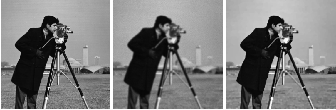
Figure 3: Result for the whole 'cameraman' image. Left : Original image of size 256 \times 256 with values scaled to [0, 3000] . Middle : Corrupted image. Right : Restoration result by the I -divergence constrained model (16) with total variation seminorm.
