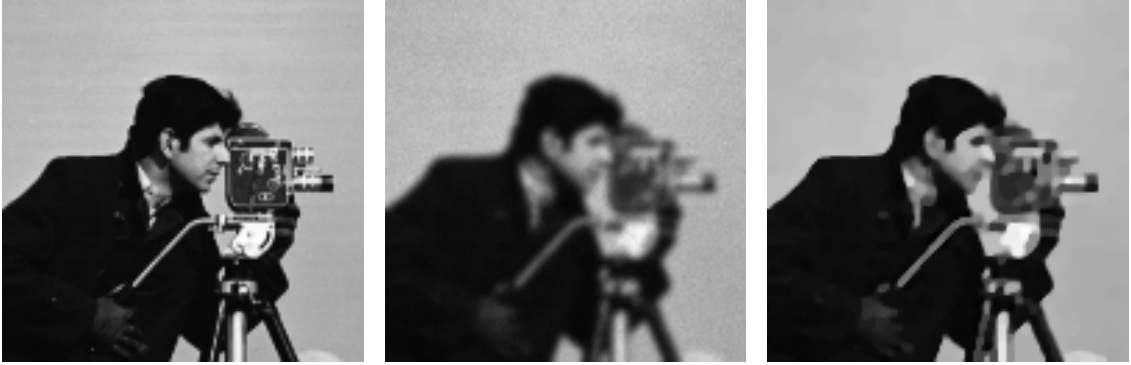
Figure 1: Left: Original image with values scaled to [0, 3000] so that the brightest pixels correspond to 3000 detected photons. Middle: Corrupted image blurred by a Gaussian kernel (standard deviation 1.3) and contaminated by Poisson noise. Right: Restoration result by the I -divergence constrained model (16) with total variation seminorm.
