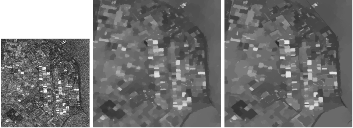
Figure 6: Left : Real multi-look SAR image (copyright by [37]) of size 512 \times 512 with values in [0, 255] . Middle : Restoration result by the I -divergence constrained model (16) with the total variation seminorm applied to the squared image. Right : Result by the I -divergence constrained model (16) with the nonlocal term ( l = 9 , \omega = 13 , a = 3 ) applied to the squared image.
