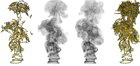
Figure 6: Simulation of a jet. Without reconnection we end up with 2560 edges after 600 simulation steps in contrast to 882 edges with reconnection. Note the almost identical structure of the particle evolutions with and without reconnections.
