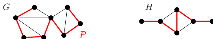
Figure 2.5: Examples: An outerhamiltonian graph G with Hamilton path P , and an outerplanar graph H which is not outerhamiltonian.
