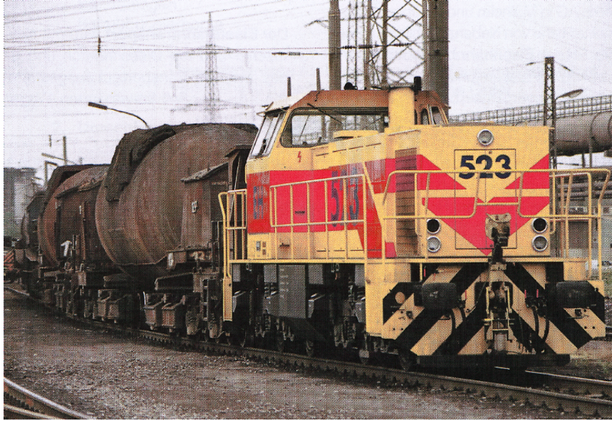
Figure1. A switching engine transports molten iron at a steel works
