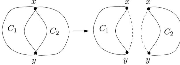
Figure 3: Removing a separating pair.
