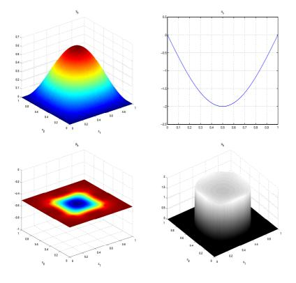
FIG. 5.1. Computed solution based on Algorithm 4.1 for h = 1/128 and  $\lambda = 10^{-7}$ : Optimal state (upper left), optimal control (upper right), adjoint state (lower left) and Lagrange multiplier (lower right).
