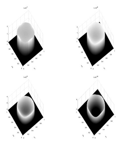
FIG. 5.2. Spurious oscillation of the Lagrange multipliers with respect to decreasing  $\lambda$ .
